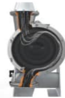
Mature impacting on the basis of the cross-current principle.
